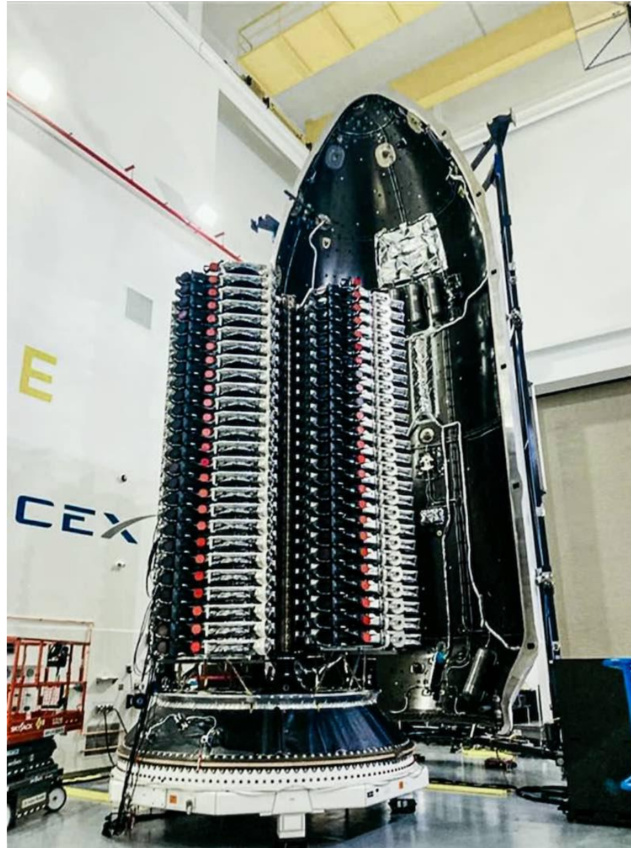
(Stack of 46 flat-packed STARLINK satellites, each about a 250kg in mass . Photo credit: SpaceX)
