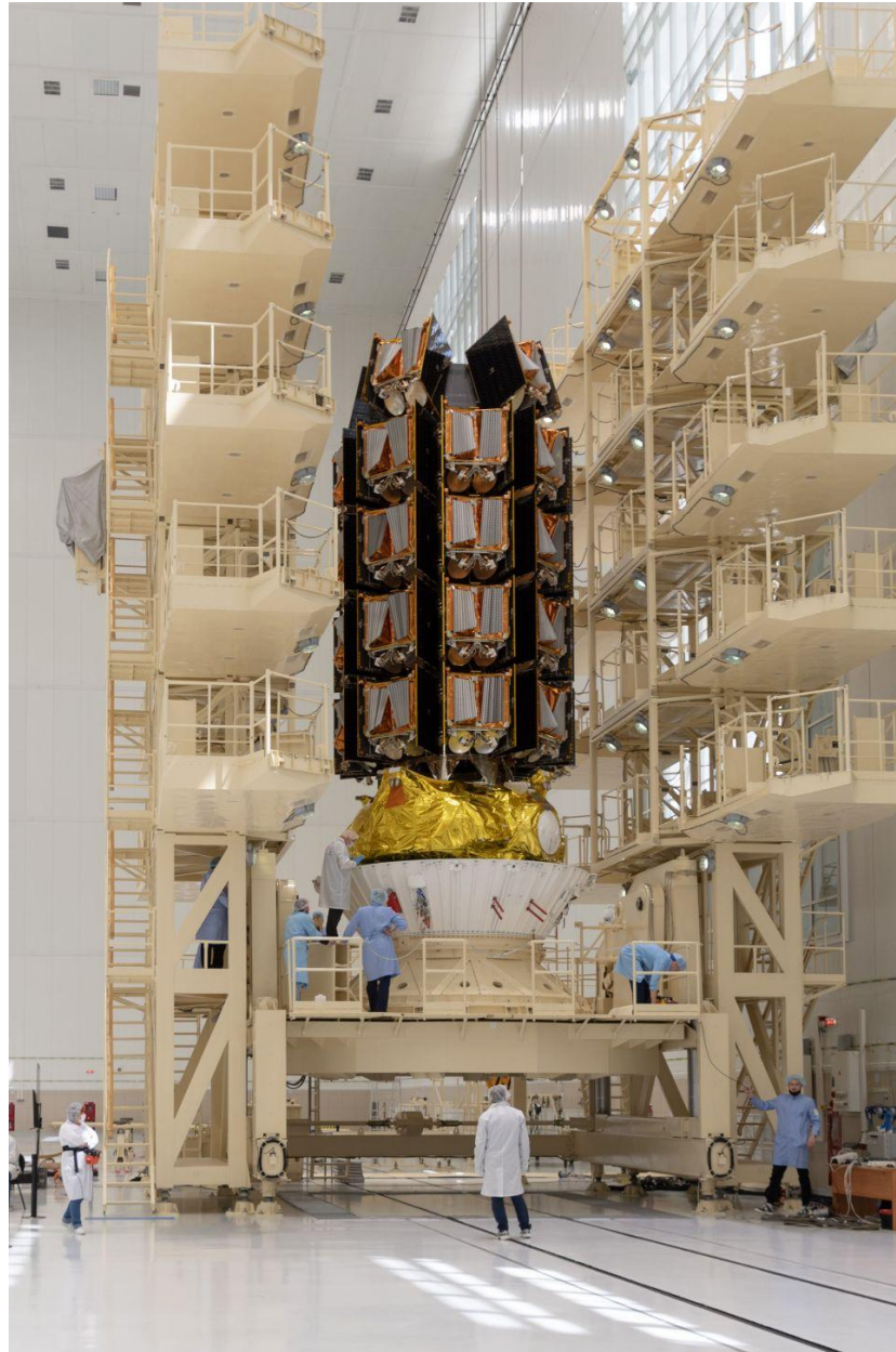
(A stack of 36 OneWeb satellites 150 kg in mass are seen in launch configuration ahead for OneWeb's launch mission. Photo credit: Arianespace)
